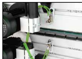
Spray station (before pre-milling or buffing)
