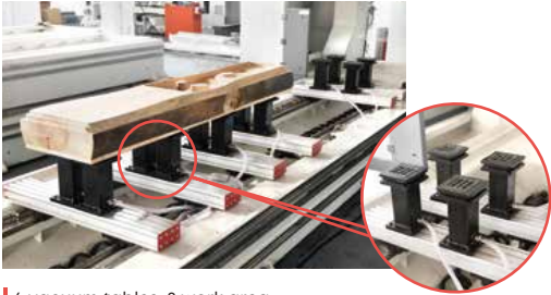
| 6 vacuum tables. 2 work area
