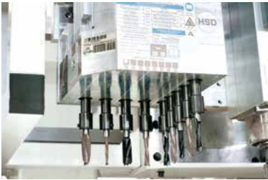
■ HQD 5+4 vertical boring block
