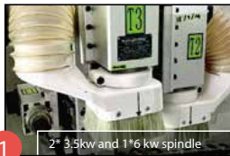
2* 3.5kw and 1*6 kw spindle
